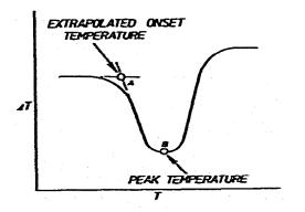
influence on the peak temperature. The extrapolated onset temperatures were marginally above the equilibrium temperatures. The standard deviations of the measured values were in the order of 5 to 8 K.
